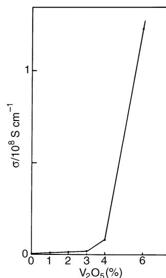
**Fig. 1** Variations in the electrical conductivity of the V<sub>2</sub>O<sub>5</sub>/TiO<sub>2</sub> samples as a function of the percentage of deposited vanadia ( $T = 250$  °C;  $P_{O_2} = 100$  Torr)
