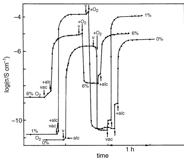
**Fig. 2** Semilogarithmic plot of the kinetics of electrical conductivity variations measured at 230 °C during various sequences in 100 Torr O<sub>2</sub> and in 45.6 Torr CH<sub>3</sub>OH (+ alc). Each sequence is separated by a brief outgassing, indicated by vac or v.
